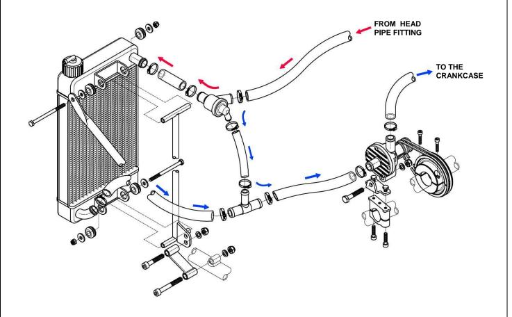
Once the system is filled (with pure water), provide to the proper air venting.
