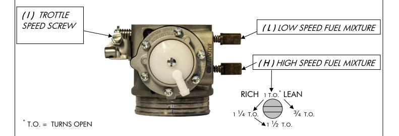
Normally the correct setting of the mixture screws, after engine run-in, is the following:
